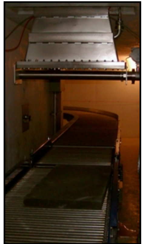
The accelerator scan horn is directed down toward the conveyer with a foam phantom on the rollers.
